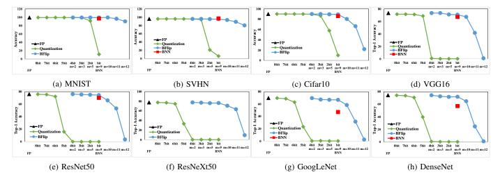
Fig. 8: Accuracy of the full-precision baseline, conventional quantization, BNN and BFlip.
