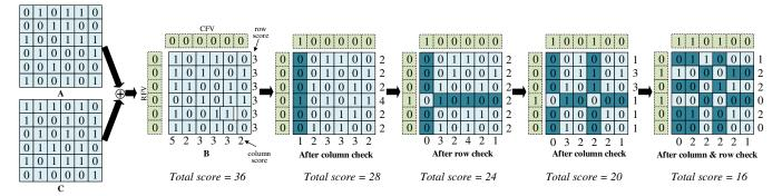
Fig. 4: Flip rows and columns to minimize the distance of two matrices. A is a bit matrix in the cluster. C is the centroid bit matrix of the cluster. B is calculated by XORing A and C.
