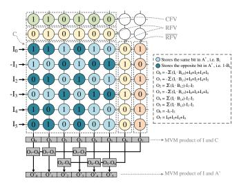
Fig. 6: Map centroid bit matrix and meta data to crossbar. *F. Mapping to Crossbars*
