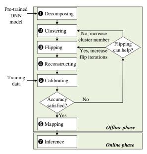
Fig. 3: The overview of BFlip's workflow.
